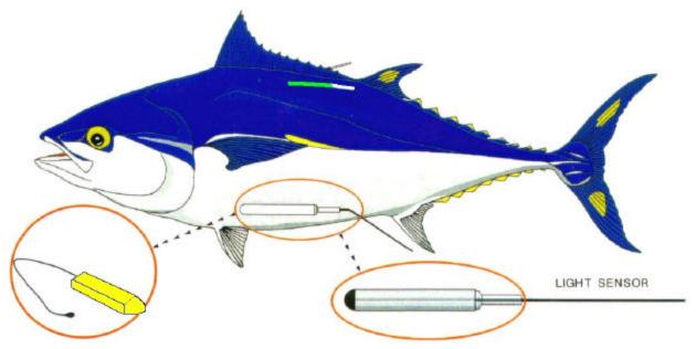
What are archival tags? Archival tags are electronic data-logging devices that provide location estimates by measuring light intensity through a light sensor. They also provide data on swimming depth, water temperature, and body temperature of the fish. This information is collected on a daily basis and stored in the tag for several years.
